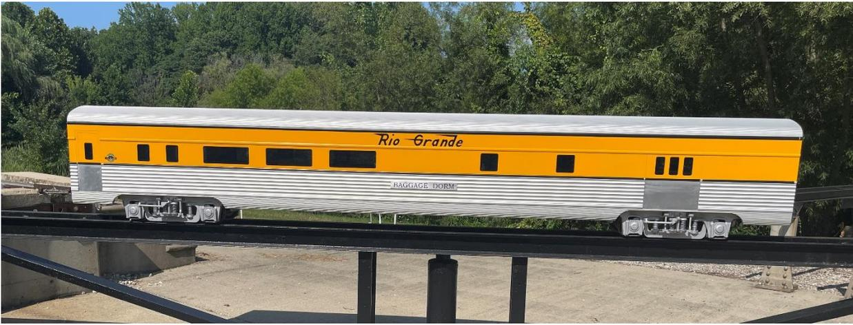
All of the 8 extruded body parts for these four DRG&W cars are fluted. The Windows can be laser or waterjet cut or conventionally milled. The entry and baggage doors are milled into the surface. Smoked Plexiglas is overlapping the window openings on the inside of the car and attached with clear silicone giving them a very clean look. There are 4 cars in this set. Built by Kent Bolerjack.
